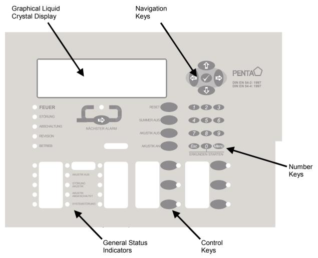
Slide-in labels are used to annotate specific General Status Indicators in addition to Function Indicators and Programmable Control Keys and Indicators.
